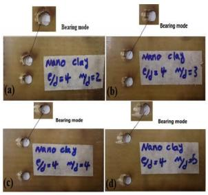
Fig. 10 Failure mode in experimental study for specimens with e/d=4 and (a): M/d=2, (b): M/d=3, (c): M/d=4, and (d): M/d=5.
