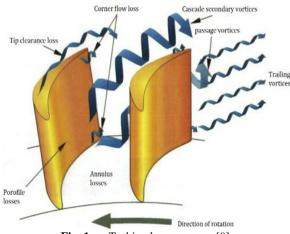
**Fig. 1** Turbine losses source [9].
