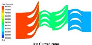
Fig. 11 Total pressure contour at 10% blade height for three modes.
