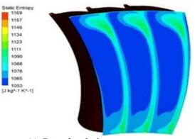
(c): Stator 2 outlet in stator curvature
