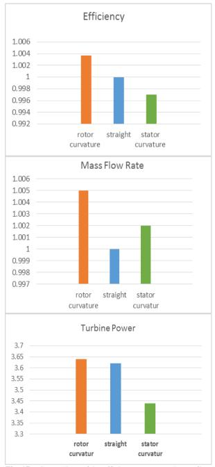
Fig. 17 Comparison of the efficiency, power and mass flow rate of the turbine.
