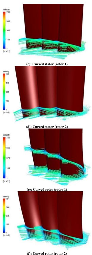
**Fig. 15** Stream lines at the hub of rotor 1 and 2.
