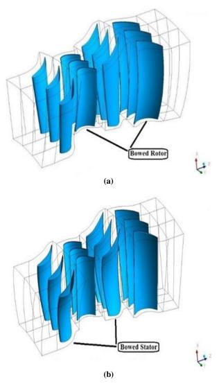
Fig. 2 Blade changes: (a): Rotors curvature and (b): Stators curvature.
