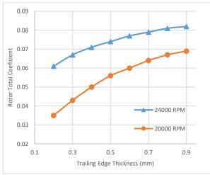
Fig. 18 Total pressure loss coefficient for rotor 1.
