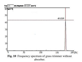
The vibrations of grass trimmer are measured using FFT vibration analyser and accelerometer mounted on the handle of grass trimmer. The vibration acceleration of grass trimmer without TVA is around 44 m/s<sup>2</sup> at handle location with operating frequency of 175 Hz and spectrum is as shown in "Fig. 10". The procedure to tune the absorber to reduce handle vibrations for different attachment location is as follows:
