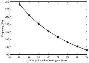
Fig. 5 Variation of frequencies of absorber with change in mass position along the rod length obtained by Dunkerleys Equation.
