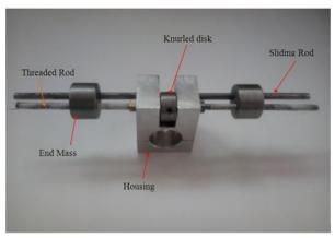
Fig. 6 Dual mass vibration absorber.
