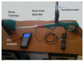
Fig. 9 Vibration measurements of grass trimmer with and without vibration absorber.
