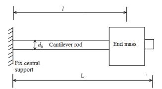
Fig. 4 Parameters of absorber used in design.
