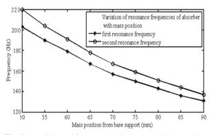
Fig. 8 Variation of frequencies of absorber with change in mass position along the rod length obtained by experimental modal analysis.
