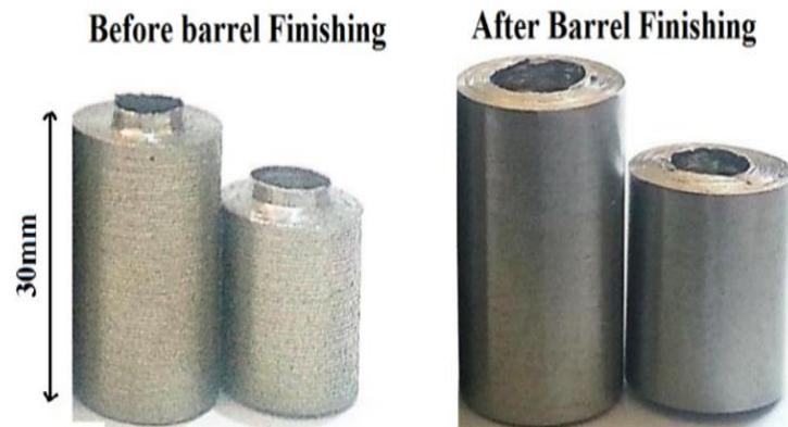
**Fig. 4** Samples before and after barrel finishing. (Working time= 2 hrs., initial roughness= 8.96 $\mu\text{m}$ , abrasive media: 75% steel balls and 25% aluminum oxide, final surface roughness= 3.75 $\mu\text{m}$ ).**Table 3** The measured surface roughness of the samples in the experiments
