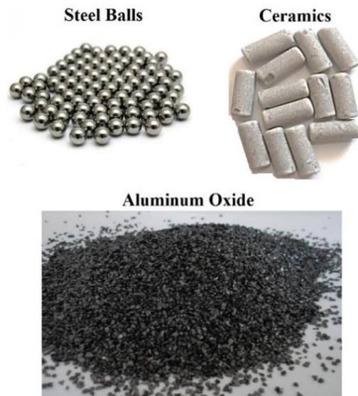
Fig. 3 Three types of used abrasive particles.
