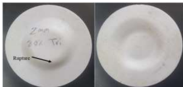
Fig. 9 Triangular pattern, density of 80%, thickness of 2 mm.
