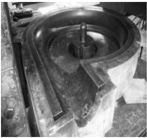
Fig. 6 Inlet liner mold for VASA HD 455-100 pump.
