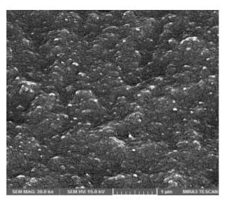
**Fig. 5** FESEM micrograph with magnification X = 30000 of NR/PBR/n-ZnO2.
