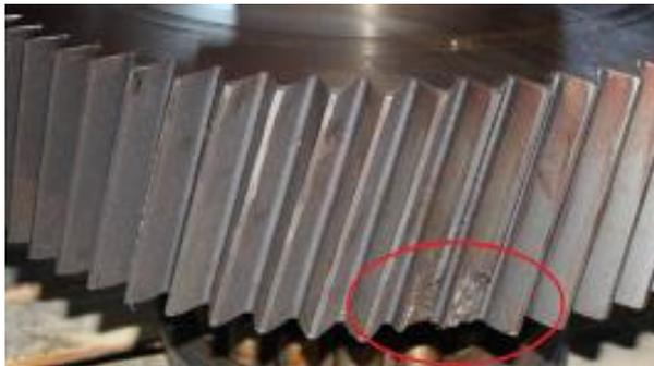
Fig. 2 Two neighbouring damaged dents on the gear
