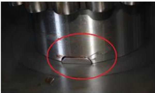
Fig. 5 Damaged location on the shaft
