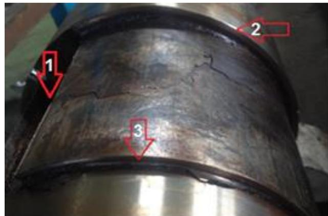
**Fig. 28** The fractured gear shaft
