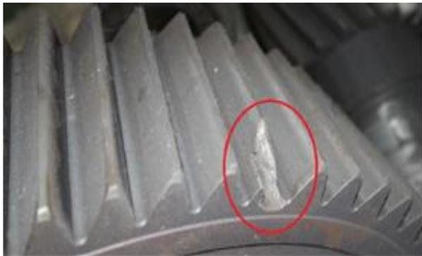
Fig. 3 The lone damaged dent on the gear
