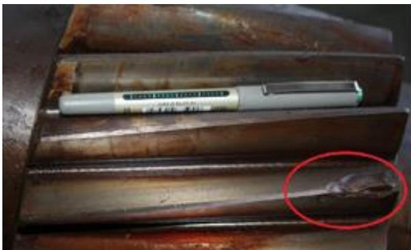
Fig. 4 The damaged dent on the pinion
