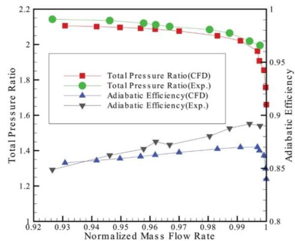
**Fig. 5** Experimental and Numerical performance map of NASA Rotor 37.
