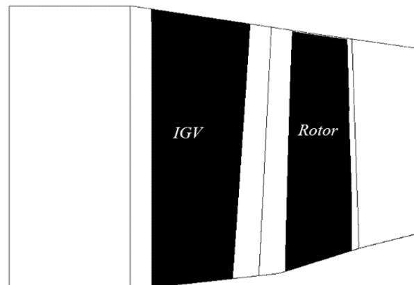
**Fig. 1** Meridional view of the IGV and the first stage rotor of axial compressor.
