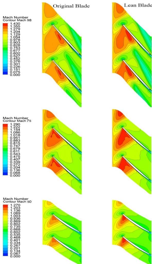
**Fig. 12** Comparison of relative Mach-number distribution at 98%, 75% and 50% of span respectively in the original and leaned blades.
