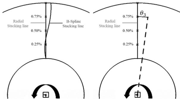
Fig. 2 Radial and B-Spline stacking line with control points.
