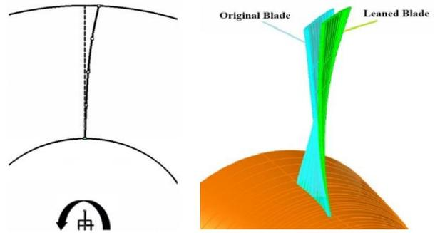
**Fig. 7** Geometrical comparison of proper leaned blade and original blade..
