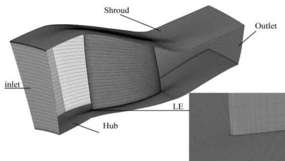
**Fig. 4** Computational grid domain of NASA Rotor 37.
