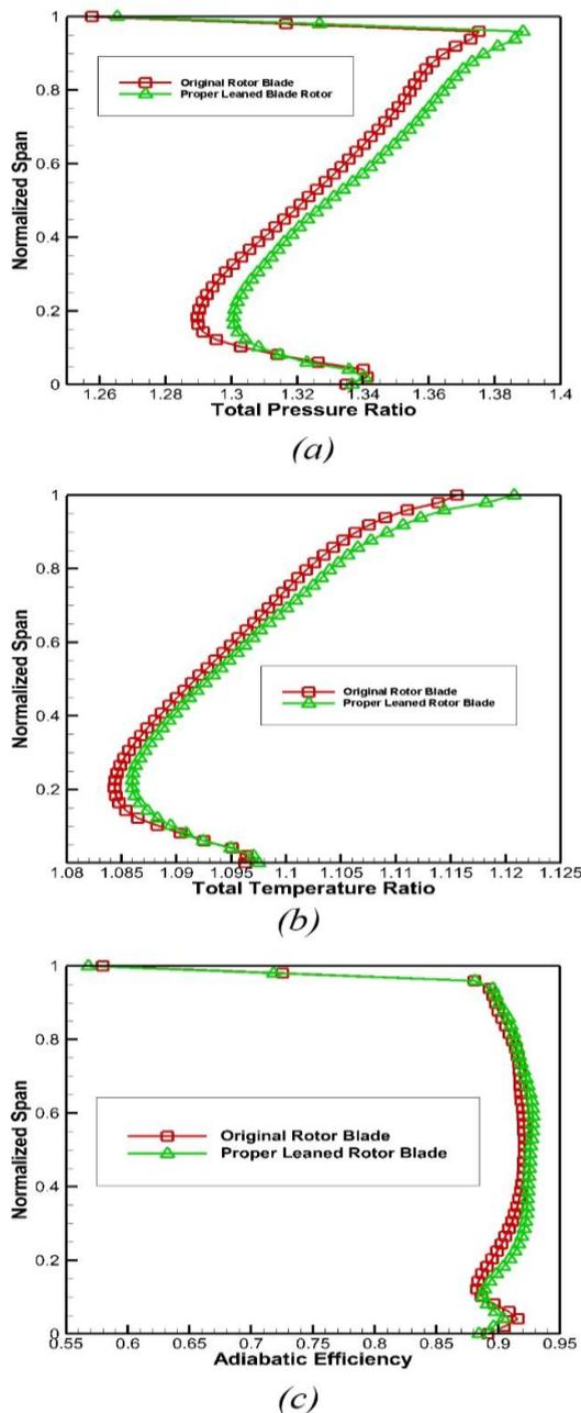
Fig. 9 Radial distributions of performance quantities at the peak efficiency condition, (a): Total pressure ratio, (b): Total temperature ratio and (c): Adiabatic Efficiency.
