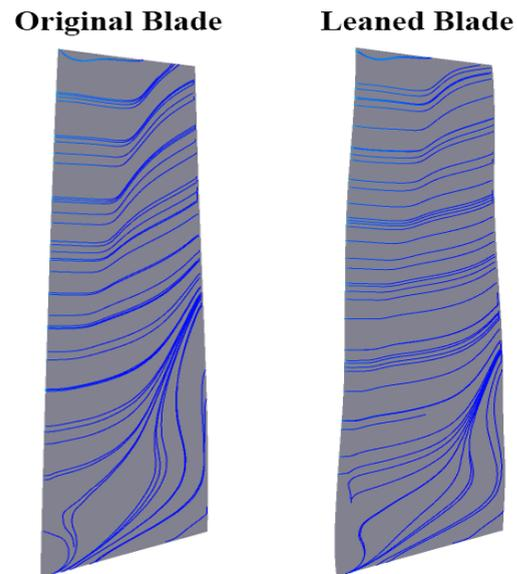
Fig. 10 Comparison of the suction surface streamlines in the original and leaned blades.
