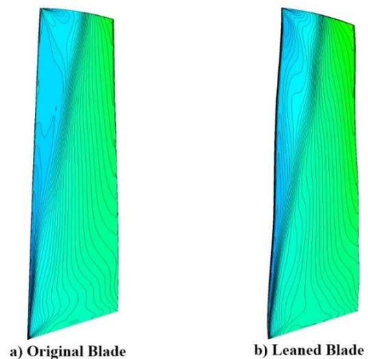
Fig. 11 Comparison of the suction surface pressure contours for original and leaned blades.
