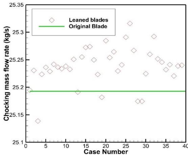
**Fig. 6** Choking mass-flow rate of different leaned blades.
