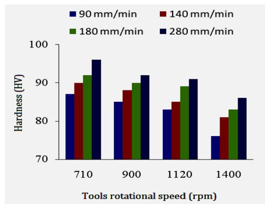
Fig. 4 Weld area Vickers hardness of samples at different tools rotational and traverse speeds
