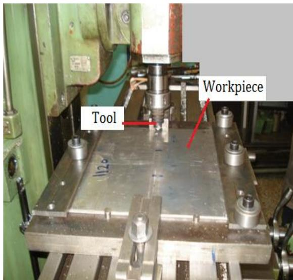
Fig. 1 FSW machine with tool and workpiece on its table
