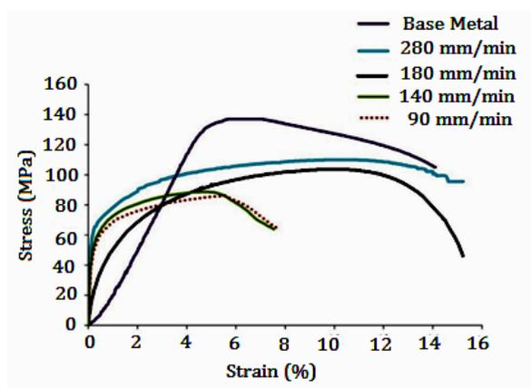
Fig. 5 Engineering stress-strain curves for base materials and welded samples in different traverse speeds (tools rotational speed = 900 rpm)
