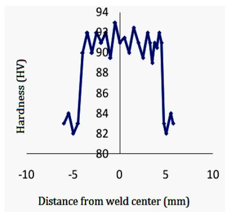
Fig. 3 Hardness curve of cross section of welded samples (tools rotational speed = 1120 rpm and traverse speed = 280 mm/min)
