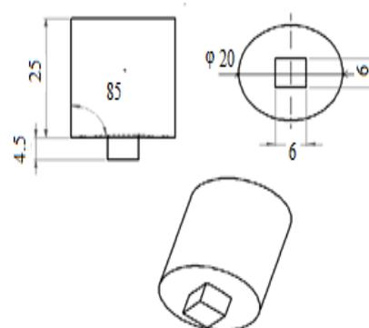
Fig. 2 (a) FSW tool used in this study, (b) schematic design of tool
