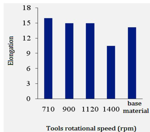
Fig. 9 Elongation of welded samples in different tools rotational speeds (traverse speed = 180 mm/min).
