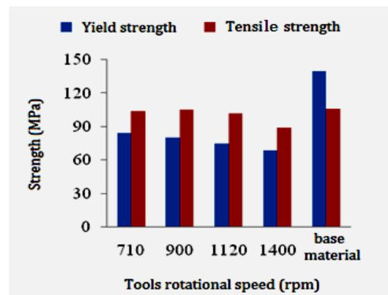
Fig. 8 Yield and tensile strength of welded samples in different tools rotational speeds (traverse speed = 180 mm/min).
