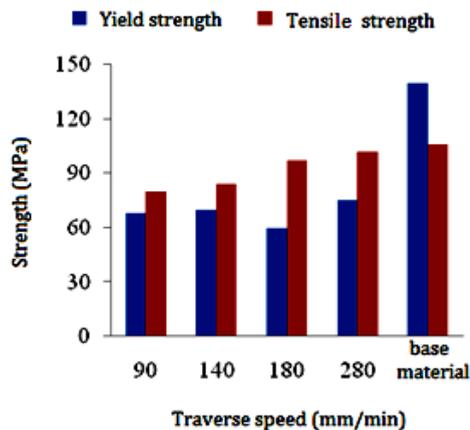
Fig. 6 Yield and tensile strength of welded samples in different traverse speeds (tools rotational speed = 1120 rpm)
