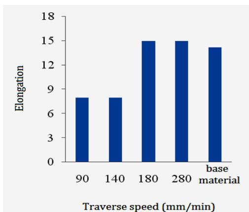
Fig. 7 Elongation of welded samples in different traverse speeds (tools rotational speed = 1120 rpm)
