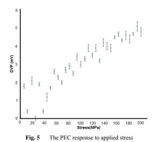
Qualitative investigation of diagram in Fig. 5 indicates that variation in applied stress on work piece results in PEC response variation. In other words, increase in applied stress leads to increase in DVP. This result is in consistency with results obtained by other researchers such as Nagy who proved that eddy current responses are directly proportional to the stress, where he used them to measure residual stresses in super alloy components [19]. However, in this study the PEC
