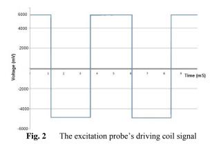
The probe's excitation frequency was set at 200 Hz. The excitation probe's driving coil signal and PEC response are shown in Figs. 2 and 3 respectively.
