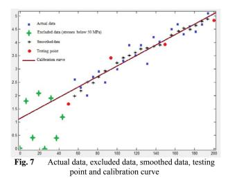
After extrapolating the calibration curve, it should be evaluated to see whether the calibration curve fits the data poorly or strongly, and to see if it is able to show data trend. In this study residual value which has been recommended for calibration curve evaluation was used as curve evaluation criterion. The residuals from a fitted model are defined as the differences between the response data and the fit to the response data at each predictor value.
