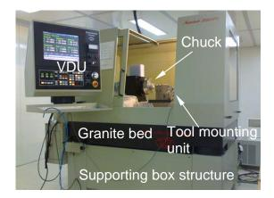
Fig. 1 Diamond Turning Machine
