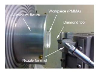
Fig. 2 Close set up view of Diamond Turning Operation
