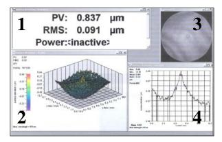
Fig. 4 Flatness Measurement of Diamond Turned Surfaces
