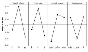
Fig. 5 Main effects plots for flatness in diamond turning of PMMA
