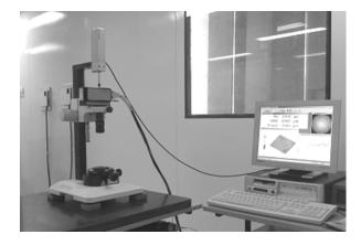
Fig. 3 Optical Interferometer for Diamond Turned Surface Measurement
