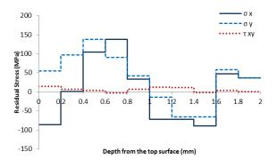
Fig. 9 Residual stress profiles  $\sigma_x$ ,  $\sigma_y$  and  $\tau_{xy}$  in the Al 5083 sample processed by ECAR
