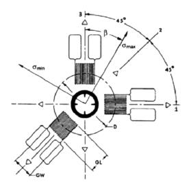
Fig. 3 Strain gauge rosette arrangement for determination of residual stress [17]
