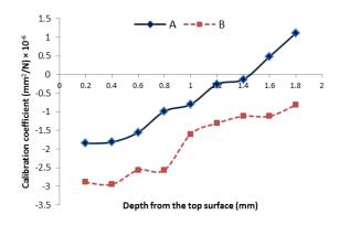
Fig. 8 Through-depth calibration coefficients  $A_n$  and  $B_n$  in ECA Red Al 5083 sample
