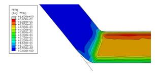
Fig. 6 The shear deformation patterns obtained by FEM calculation
