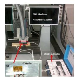
**Fig. 5** (a) High speed drilling set up of relieved strains (b) The gauge rosette bonded to the surface of ECARed sample
