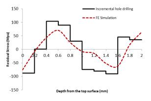
Fig. 10 Results comparison for the Incremental hole drilling and FE simulation
