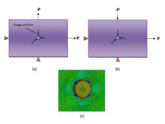
Fig. 4 Two types of loading applied on the model to obtain (a) calibration coefficients  $A_n$ , (b) calibration coefficients  $B_n$  and (c) strain result of FE simulation under loading
