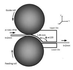
Fig. 1 Schematic representation of the ECAR process
