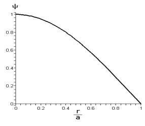
Fig. 2 Dimensionless deflection for pinned plate
