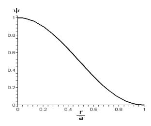
Fig. 3 Dimensionless deflection for clamped plate
