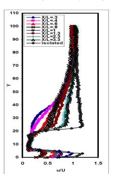
Fig. 7 Mean velocity profiles in the wake of the car subjected to the wake of the trailer(x/l=0.01)
