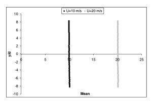
Fig. 3 Average speed fluctuation in the wind tunnel for speeds of 10 and 20 m/s
