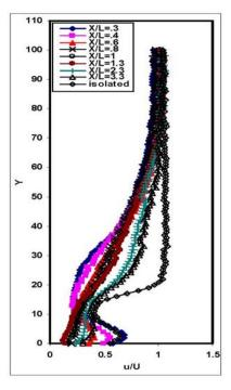
Fig. 9 Mean velocity profiles in the wake of the car subjected to the wake of the trailer(x/l=0.5)
