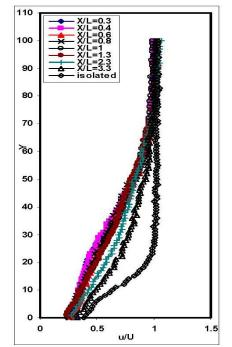
Fig. 13 Mean velocity profiles in wake of car subjected to wake of trailer (x/l=1.5)
