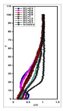
**Fig. 10** Man velocity profiles in the wake of the car subjected to the wake of the trailer(x/l=0.75)
