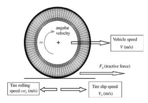
Fig. 2 Free body diagram of a single tire
