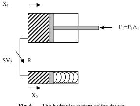
The hydraulic system of the device Fig. 6
