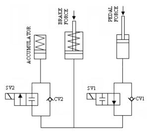
Fig. 4 The diagram of motorcycle new ABS hydraulic circuit
