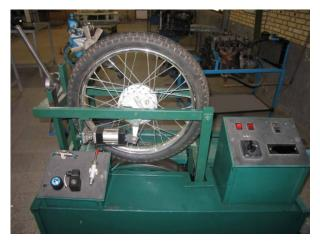
**Fig. 1** The new ABS and its pilot model
