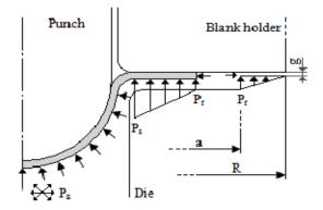
**Fig. 3** The fluid pressure distribution on the flange area during the forming process [22]
