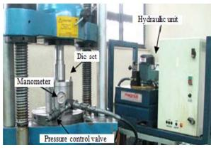
Fig. 4 Experimental equipment and the manufactured die set
