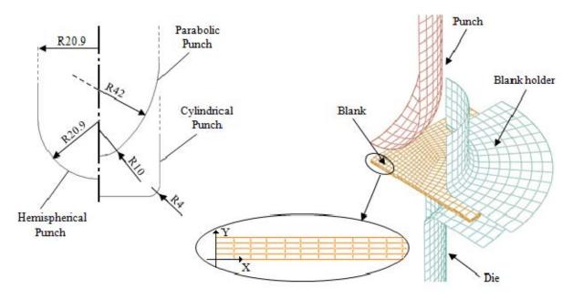
Fig. 2 The exploded view of the FEM models (one-quarter geometry).
