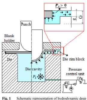
**Fig. 1** Schematic representation of hydrodynamic deep drawing assisted by radial pressure.
