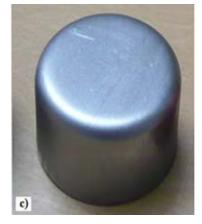
Fig. 5 Photograph of the hydroformed work pieces obtained from experiments (a) parabolic cup, (b) hemispherical cup, (c) cylindrical cup
