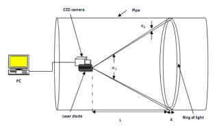
Fig. 1 Schematic view of the optical system
