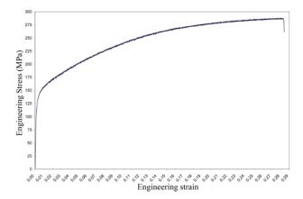
Fig. 2 Engineering stress-strain diagram for Cu C11000
