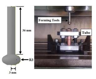
**Fig. 3** (a) the forming tool, (b) experimental setup
