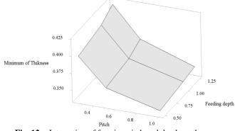
Fig. 12 Interaction of forming pitch and depth on the minimum thickness
