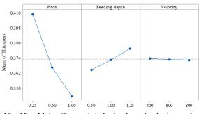
Fig. 10 Main effects of pitch, depth, and velocity on the thickness
