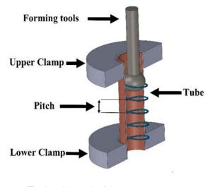
Fig. 1 Schematic of the process components
