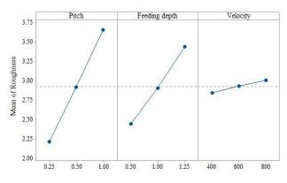
Fig. 7 Main effect plots of pitch, feeding depth and tool velocity on surface roughness
