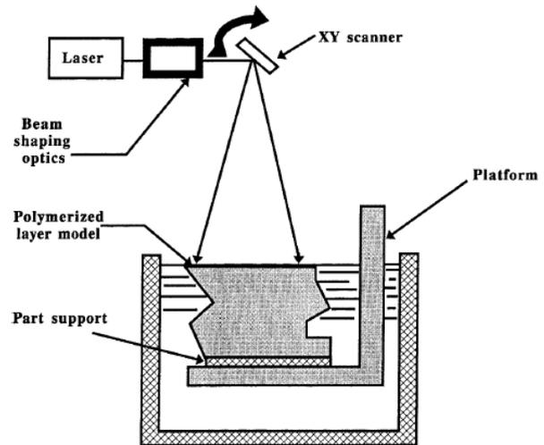
Fig. 1 Schematic view of a SLA machine
