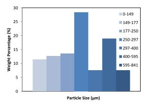
Fig. 1 Particle size distribution of wood
