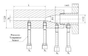
Fig. 2 Schematic picture of the utilized extrusion dies showing the locations of the temperature-pressure sensors (dimensions are in mm)
