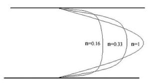
Fig. 3 Velocity profiles for melts with different power law indexes [28]
