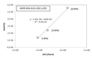
**Fig. 7** Volumetric flow rate vs.  $\Delta P/L$  for the composite containing HDPE5620 as the polymer matrix and 50wt% of wood content (Die temperature: 155°C, die length to diameter ratio: 5, die diameter: 10mm)
