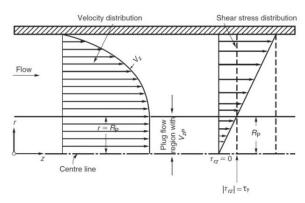
**Fig. 4** Schematic velocity distribution for laminar flow of a Bingham plastic fluid in a pipe [29]
