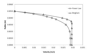
**Fig. 8** Suggested velocity distributions for wood plastic composite with HDPE5620 as the polymer matrix and 50 wt% wood content, based on Power law and Bingham plastic models
