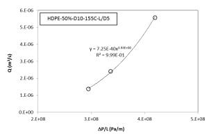
**Fig. 6** Volumetric flow rate vs.  $\Delta P/L$  for the composite containing HDPE5620 as the polymer matrix and 50wt% of wood content (Die temperature: 155°C, die length to diameter ratio: 5, die diameter: 10mm)
