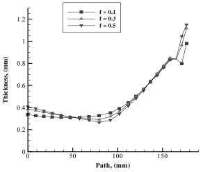
Fig. 5 Comparison of thickness distribution in  $5 \times 10^{-4}$  s<sup>-1</sup> strain rate and different friction coefficients
