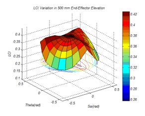
**Fig. 6** Local Conditioning Index versus EE orientation in z=500mm
