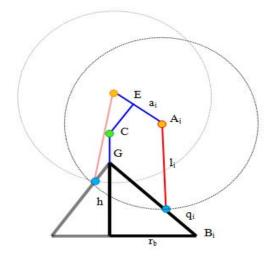
Fig. 3 Schematic configuration of 3-CRS kinematic
