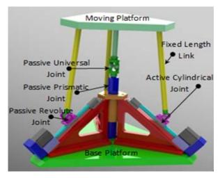
Fig. 1 CAD model of 3-CRS/PU parallel manipulator
