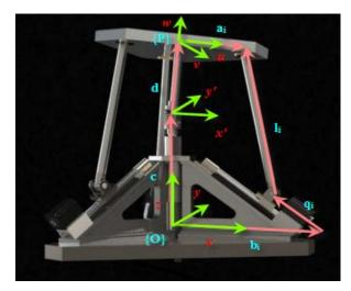
Fig. 2 Geometrical Model of 3-CRS/PU
