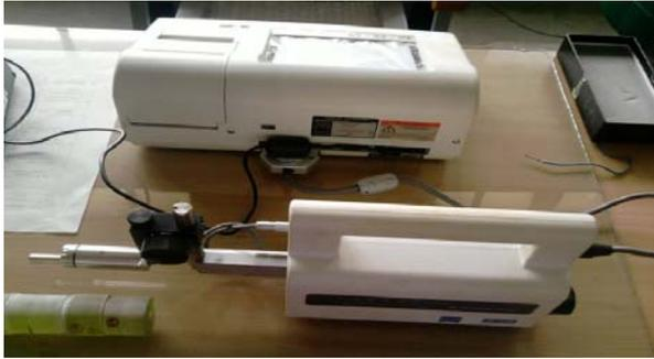
**Fig. 2** Surface Roughness Tester: Tokyo Seimitsu Surfcom 130A
