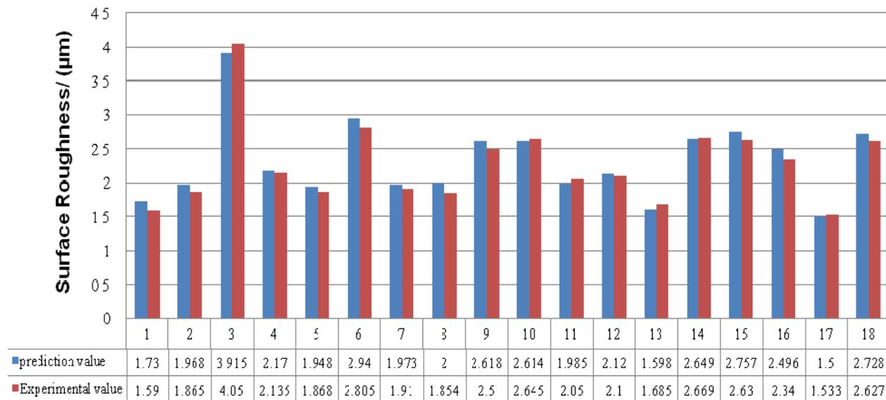
Fig. 5 Comparison between actual and predicted values of surface roughness
