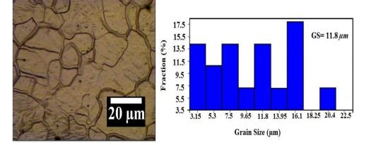
Fig. 2 Microstructure and histogram of grain size distribution for wire with the rotational speed of 250 rpm; vertical speed of 20 mm/min, and extrusion hole size of 5 mm.
