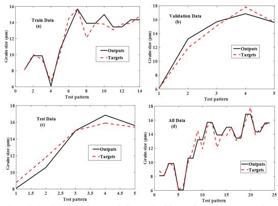
**Fig. 6** The actual and predicted values of average grain size: (a): The training step, (b): Validation step, (c): Testing step and (d): All steps together.
