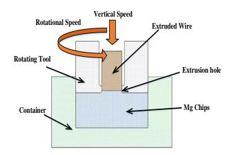
Fig. 1 Schematic of friction stir extrusion setup.
