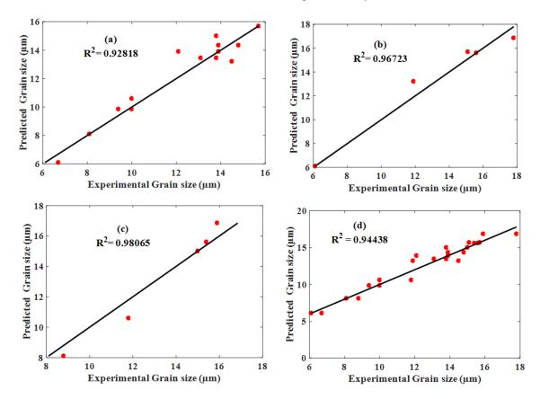
Fig. 7 Correlation between actual and predicted data at: (a): training step, (b): validation step, (c): test step and (d): all steps together.
