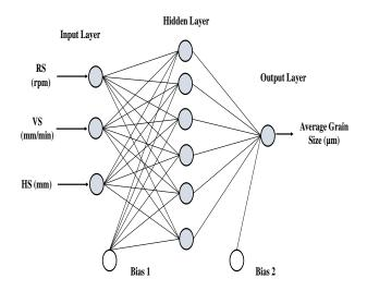
Fig. 4 Schematic of the current three–layer neural network.
