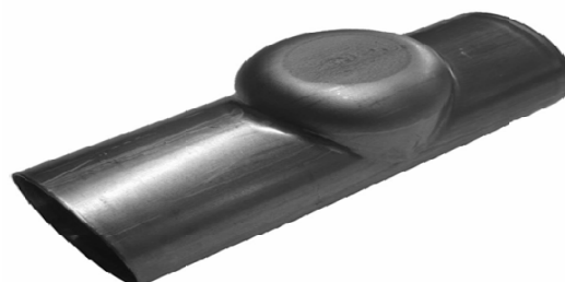
Fig. 8 Result of experimental test in T-shape hydro-formed part
