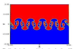
**Fig. 11** Patchy Structure of the branches of nonlinear RT instability by accelerating heavy fluid (blue) into lighter fluid (red) at the time of T=1.5 (sec)
