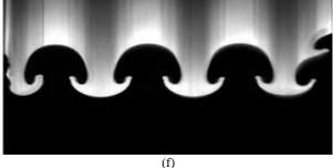
Fig. 3 (part 2) The behaviour of the fluid interface given an initial sinusoidal disturbance is experimentally shown to be unstable under constant downward acceleration of g [8]
