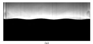
**Fig. 3** (part 1) The behaviour of the fluid interface given an initial sinusoidal disturbance is experimentally shown to be unstable under constant downward acceleration of g [8]
