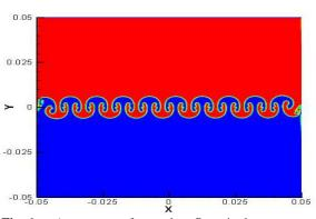
**Fig. 6** Appearance of secondary flows in the structure of vortices by further development of the heavy fluid (blue) into lighter fluid (red) at the time of T=1.0 (sec)
