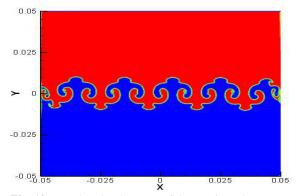
**Fig. 10** Further development of the quasi-mushroom type RT instability by accelerating heavy fluid (blue) into lighter fluid (red) at the time of T=1.0 (sec)
