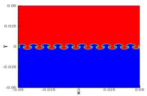
**Fig. 5** Formation of mushroom type RT instability by accelerating heavy fluid (blue) into lighter fluid (red) at the time of T=0.5 (sec)
