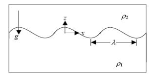
**Fig. 2** Schematic of a sinusoidal disturbance at the interface of two constant densities media in a closed chamber
