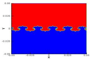
Fig. 9 Formation of quasi-mushroom type RT instability by accelerating heavy fluid (blue) into lighter fluid (red) at the time of T=0.5 (sec)
