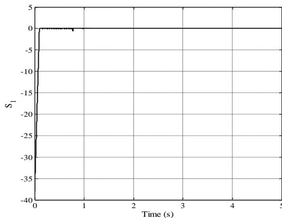
Fig. 2 The sliding surface of the sliding mode controller for the Lorenz chaotic problem.
