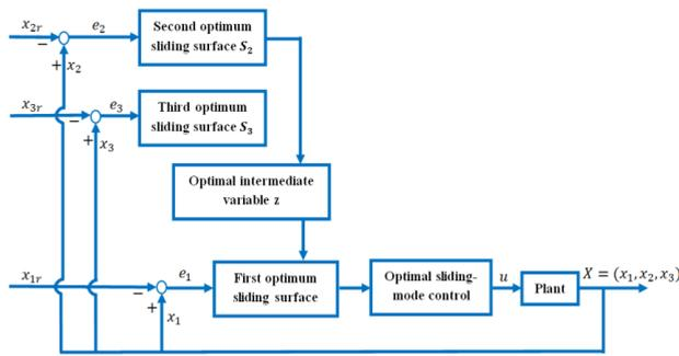
Fig. 8. The block diagram of the optimum sliding-mode control system for the Lorenz chaotic problem.
