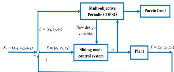
**Fig. 6** The block diagram to find the Pareto front of the sliding-mode control for the Lorenz chaotic problem based on the multi-objective periodic CDPSO algorithm.
