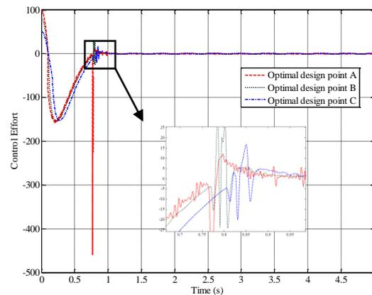
Fig. 12. Control effort of the optimum design points A, B, and C shown in the Pareto front.
