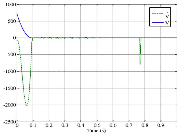
Fig. 1 Lyapunov function and its derivative to show the asymptotical stability of the system.
