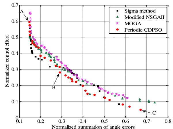
**Fig. 7.** The obtained Pareto fronts by using Sigma method [45], Modified NSGAI [76], MOGA (MATLAB Toolbox), and the proposed algorithm for the optimal control of the Lorenz chaotic problem.
