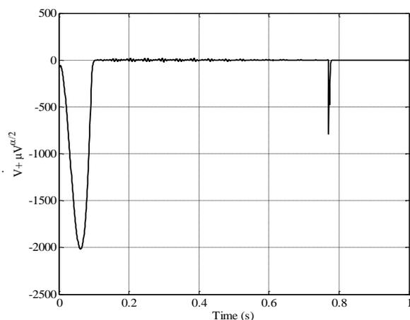
Fig. 5  $\dot{V}(x) + \mu(\sqrt{V})^\alpha$  is always negative and the state errors will be attained in finite time.
