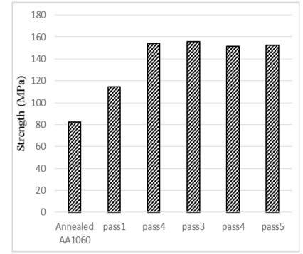
Fig. 4 Variations of the strength value of AA1060/ Al<sub>2</sub>O<sub>3</sub> composites with the Warm-ARB passes
