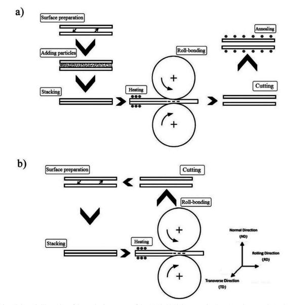
Fig. 1 Schematic illustration of the production process of the AA1060/ Al<sub>2</sub>O<sub>3</sub> composite sheet (a): primary cycle (cycle#0) and (b): main cycles
