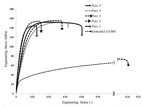
Fig. 3 Engineering stress-strain tensile test curves for Al/ Al<sub>2</sub>O<sub>3</sub> composites before and after Warm-ARB
