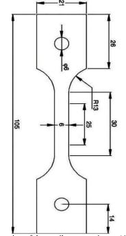
**Fig. 2** Orientation of the tensile test specimens (ASTM-E8M), [18]
