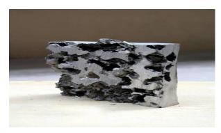
Fig. 5 Soaked Precursors at 850°C (using aluminum net)
