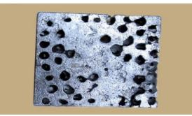
Fig. 9 Porous casting at 950°C
