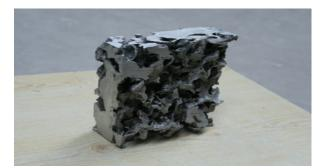
Fig. 6 Soaked Precursors at 850°C (using steel net)
