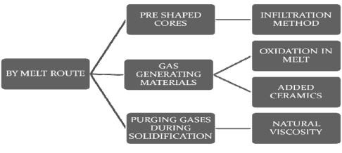
Fig. 1 Melt route methods for production of metal foams
