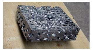
Fig. 10 Porous castings at 910°C
