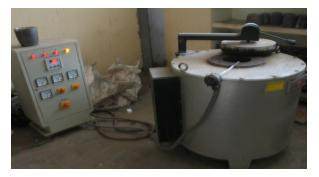
Fig. 2 Electrically heated crucible furnace
