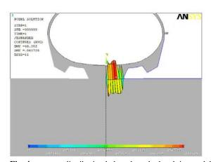
**Fig. 4** stress distribution below the calculated tire model. It shows analyzed stress distribution similar to the pattern measured by (T. Keller, 2005) and (Arvidsson et al., 2002). and the Sohne model.
