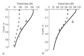
Fig. 3 Measured vertical stress (triangles) for a wheel load of 81.6 kN, and a tire inflation pressure of (a) 90 kPa and (b) 220 kPa; and calculated stress according to Sohne (1953) assuming a circular contact area with a uniform stress distribution (broken curves) and using generated contact stress distribution according to the proposed model (solid curves); measured values from Arvidsson et al. (2002) [12].
