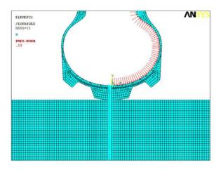
Fig. 1 Developed uniform 150 kPa inflation pressure without vertical load
