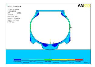
Fig. 2 Stresses after 150 kPa inflated tire with uniform inflation pressure
