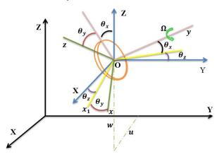
Fig. 2 Rotating frames of a disc on a rotating flexible shaft
