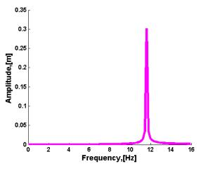
Fig. 6 Maximum response of the simple rotor in the present study
