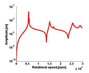
Fig. 9 Frequency response of the rotor of example 4 in the present study for point 6
