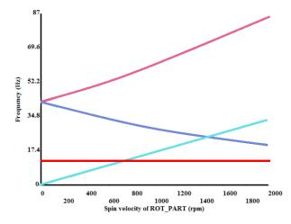
Fig. 3 Campbell's diagram of the rotor using Ansys [16]
