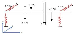
Fig. 1 A general model of the rotor-bearing system with arbitrary conditions.
