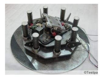
**Fig.1** The stabilometer used in the study without outer frame and upper plates
