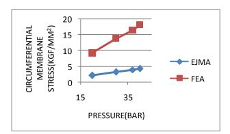
Fig. 5 Circumferential stresses in bellow tangent ( $S_1$ ) for Inconel 625. $S_1 < S_{ab}(21 \text{ kgf/mm}^2)$
