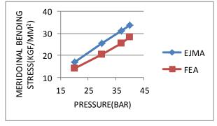
Fig. 9 Meridional bending stress (S<sub>4</sub>) for Inconel 625  $(S_3+S_4) < C_m \times S_{ab} (63 \text{ kgf/mm}^2)$
