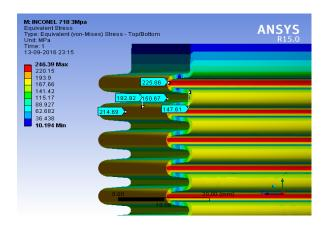
Fig. 20 Stress distribution at Pressure 30 Bar
