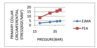
**Fig. 6** Primary collar circumferential stress  $(S_1^{-1})$  for Inconel 625. $S_1^{-1} < S_{ab}$  (21 kgf/mm<sup>2</sup>)
