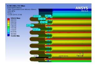
Fig. 22 Stress distribution at Pressure 40Bar
