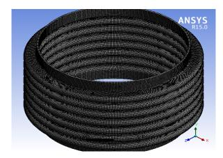
Fig. 3 The meshed model
