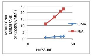
Fig. 8 Meridional membrane stress (S<sub>3</sub>) for Inconel 625
