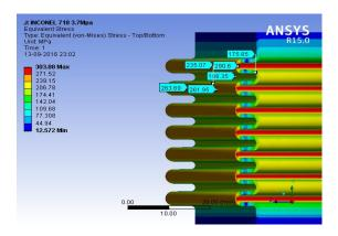
Fig. 21 Stress distribution at Pressure 37 Bar
