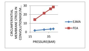
Fig. 16 Circumferential membrane stress induced in convolution ( $S_2$ ) for Inconel 718  $S_2$  <  $S_{ab}$  (32.34 kgf/mm<sup>2</sup>)
