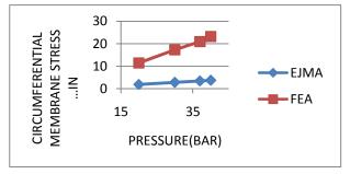
Fig. 7 Circumferential membrane stress induced in convolution ( $S_2$ ) for Inconel 625  $S_2 < S_{ab}$  (21 kgf/mm<sup>2</sup>)
