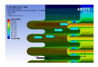
Fig. 12 Stress distribution at pressure 37 Bar
