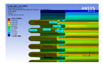
Fig. 10 Stress distribution at pressure 20 Bar
