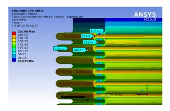
Fig. 11 Stress distribution at pressure 30 Bar
