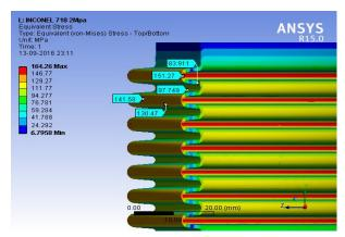
Fig. 19 Stress distribution at Pressure 20 Bar
