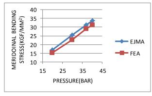
$\begin{array}{ll} \textbf{Fig. 18} & \text{Meridional bending stress } (S_4) \text{ for Inconel} \\ 718(S_3 + S_4) & <\!C_m \! \times \! S_{ab} (97.02 \text{ kgf/mm}^2) \end{array}$
