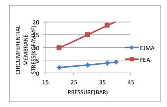
Fig. 14 Circumferential stresses in bellow tangent  $(S_1)$  for Inconel  $718S_1 < S_{ab}(32.34 \text{ kgf/mm}^2)$
