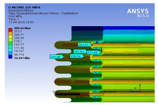
Fig. 13 Stress distribution at pressure 40 Bar
