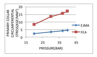
Fig 15 Primary collar circumferential stress  $(S_1^{-1})$  for Inconel  $718S_1^{-1} < S_{ab} (32.34 \text{ kgf/mm}^2)$
