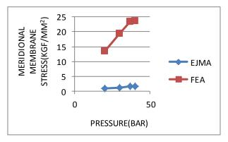
**Fig. 17** Meridional membrane stress (S<sub>3</sub>) for Inconel 718
