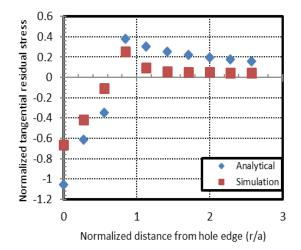
**Fig. 8** Comparison of tangential residual stress on entrance plate of mandrel in movement by 1.5% degree of expansion
