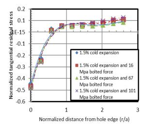
Fig. 9 Tangential residual stress field distribution in cross section and changes after closing bolts by three different pressure forces in mandrel entrance plate
