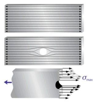
Fig. 2 Stress distribution around the hole [15]
