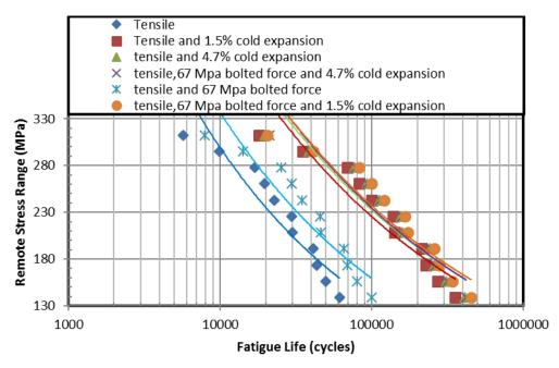
Fig. 14 The S-N diagram for Al 2024-T3 with bolt load 67 MPa
