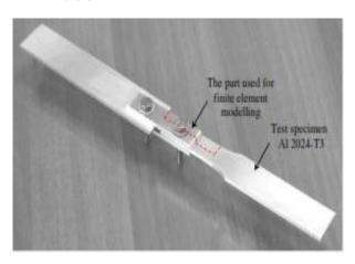
Fig. 11 The fixture used in the tests and the part used for finite element modeling [8]
