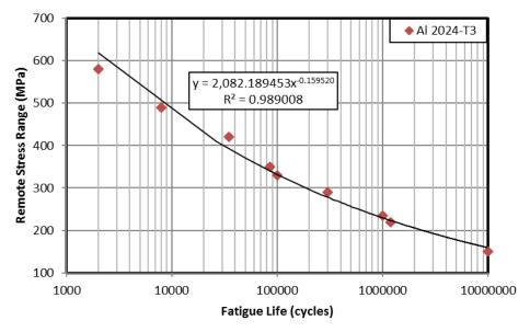
Fig. 13 The S-N diagram for Al 2024-T3
