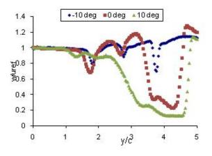
**Fig. 6** Comparison of dimensionless mean velocities at 3 different attack angles (cascade in presence of tripping wires)
