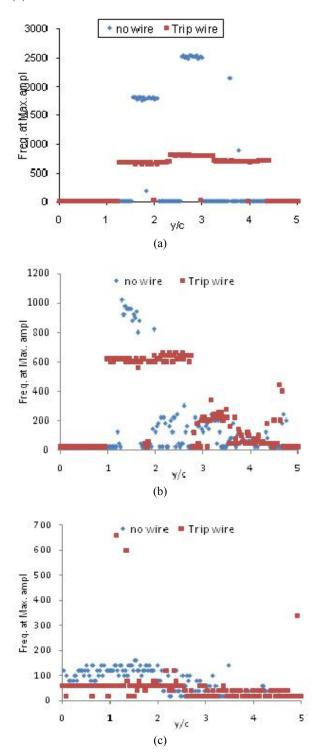
**Fig. 12** Comparison of flow frequency at the maximum amplitude for cascade in the presence and absence of tripping wires at different attack angles: a) I=-10, b) I=0, c)I =10
