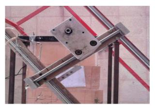
Fig. 2 location of probe displacing system on compressor cascade
