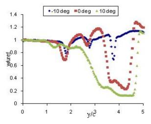
**Fig. 5** Comparison of dimensionless mean velocitiesat 3 different attack angles (tripping wires-free cascade)
