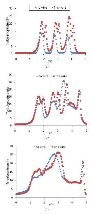
**Fig. 10** Comparison of turbulence intensities of cascade in presence and absence of tripping wires at different attack angles: a) I =-10, b) I =0, c) I =10
