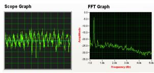
Fig. 11 Flow oscillation in time domain on left and in frequency domain on the right
