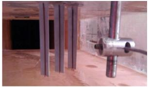
Fig. 3 Placingtripping wires on compressor's blades in wind tunnel
