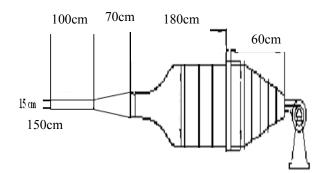
Fig. 1 Wind tunnel schematic andvessel experimental setup
