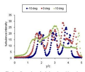
Fig. 9 Comparison of turbulence intensities at three different attack angles (cascade in the presence of tripping wires)
