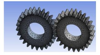
Fig. 1 The meshed model of Spur gear
