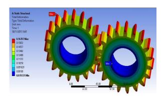
Fig. 9 Total deformation on Al 6061-T6
