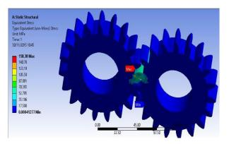
Fig. 2 The equivalent Stress on Al 7050-T7451
