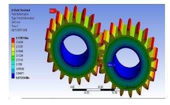
Fig. 7 Total deformation on Al 6106-T6
