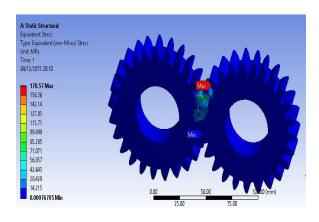
Fig. 4 Equivalent Stress on Al 7075-T651
