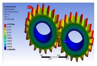
Fig. 3 Total deformation on Al 7050-T7451
