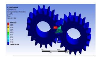
Fig. 8 The equivalent stress on Al 6061-T6
