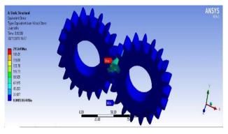
Fig. 6 The equivalent Stress on Al 6106-T6
