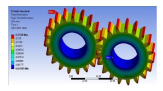
Fig. 5 Total deformation on Al 7075-T651
