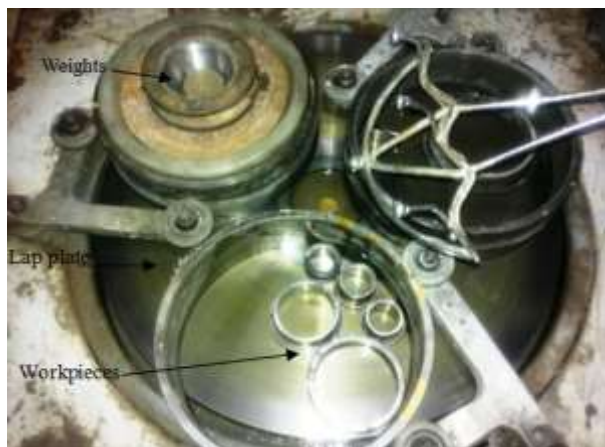
Fig. 1 The Lapping process
