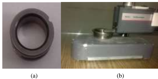
Fig. 2 a) The workpiece, b) Surface roughness measurement
