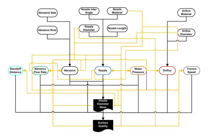
Fig. 3 Relation between different parameters in AWJ machining process
