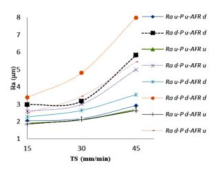
Fig. 5 Diagram of the surface roughness to the TS ( $P_u$ =3800 bar &  $P_d$ =3500 bar and AFR<sub>u</sub>=400 g/min & AFR\_d=300 g/min)
