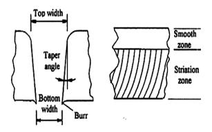
Fig. 2 Schematic and definition of kerf geometry [6]
