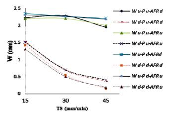
Fig. 4 Diagram of kerf width in the upper and lower sections relation the TS ( $P_u$ =3800 bar &  $P_d$ =3500 bar and AFR<sub>u</sub>=400 g/min & AFR\_d=300 g/min)
