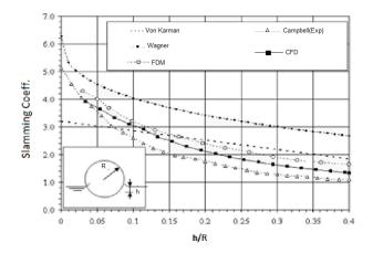
Fig. 5 Variation of slamming coefficient to (h/R) [13]
