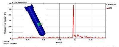
Fig. 14 Variations of shear stress versus time for an element in the middle of the mine
