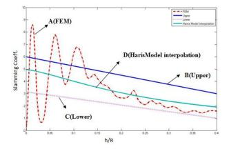
Fig. 4 Variation of slamming coefficient to (h/R)
