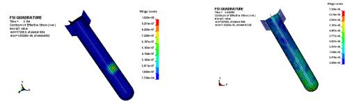
Fig. 12b Contour of Von Mises stress variation for the mine colliding with water at two different times
