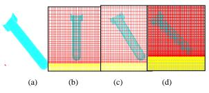
Fig. 9 Finite element model, a) Mine elements, b) Water and air elements with  $90^0$  mine impact angle, c)  $60^0$  mine impact angle, d)  $45^0$  mine impact angle
