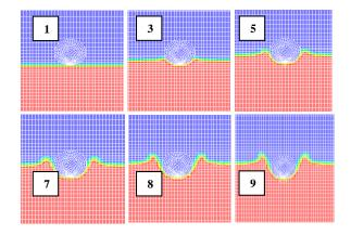
Fig. 7 Variations of water surface in cylinder impact at six different times (simulation by Ls-Dyna)
