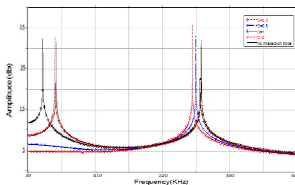
**Fig. 4** Vibration amplitude of vertical displacement in air environment in repulsive region
