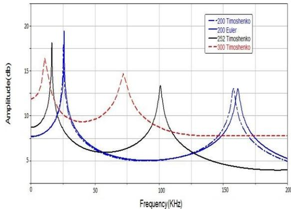
**Fig. 12** The amplitude of vertical displacement versus the frequency in liquid environment at different cantilever lengths
