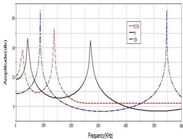
**Fig. 9** The effect of cantilever height on the amplitude of vertical displacement in air environment
