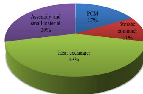
Fig. 10 Total cost break down of the storage system
