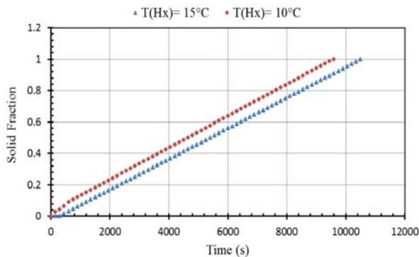
Fig. 7 Solid fraction distribution versus time in solidification process
