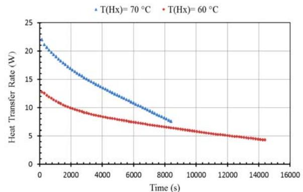
Fig. 6 Heat transfer rate versus time in melting process
