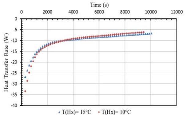
Fig. 9 Heat transfer rate as function of time in solidification process
