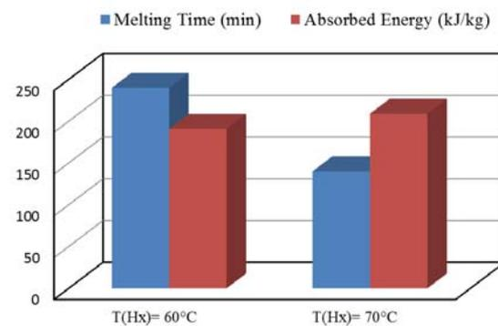
Fig. 5 Comparison of total melting time and total quantity of heat absorbed for different configuration
