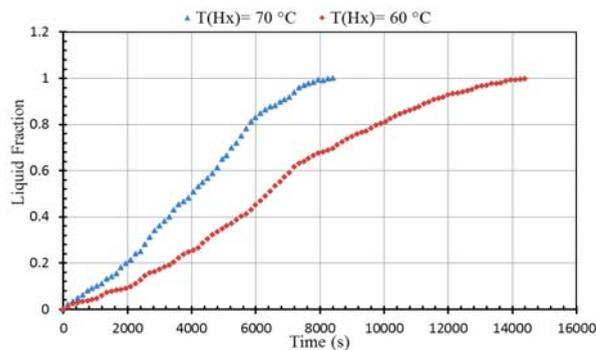
Fig. 3 Liquid fraction distribution versus time in melting process
