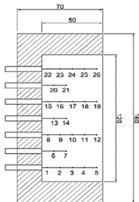
Fig. 2 Thermocouple arrangement in a storage container
