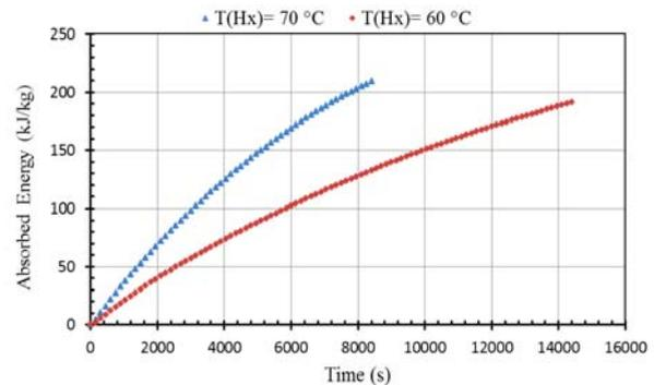
Fig. 4 Absorbed energy versus time in melting process
