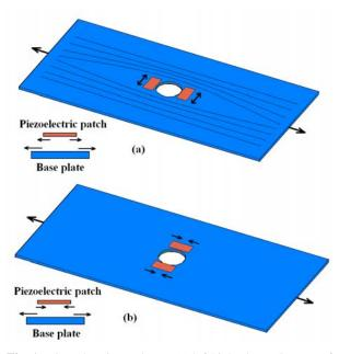
Fig. 1 Piezoelectric patches at (a) left/right (b) top/bottom of the hole
