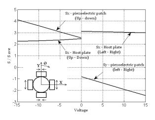
Fig. 9 Comparison of the stress around the hole regarding placements of piezoelectric patches at left/right and top/bottom of the hole
