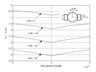
Fig. 8 Distribution of Sy in piezoelectric patches for left/right location of patches
