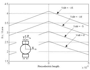
Fig. 5 Distribution of Sx in piezoelectric patches for top/bottom location of hole
