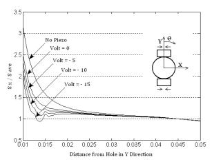
Fig. 4 Distribution of Sx along the X axis of plate for top/bottom location of patches
