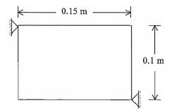
Fig. 4 Diagonally Supported Rectangular Plate [11]
