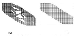
Fig. 5 Optimal designs of rectangular plate for First natural frequency; material removed, 50% (A) [11], (B) BCO Method
