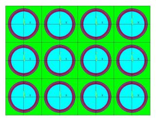
Fig. 1 Transverse cross-section of the 1-D unidirectional C/SiC composites
