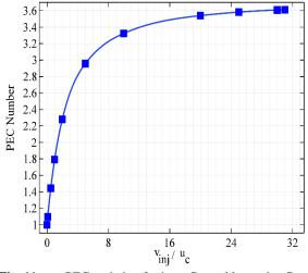
**Fig. 11** PEC variation for input Reynolds number Re =  $1, \phi = 0.02, B = 0.1$ , and different injection velocities.
