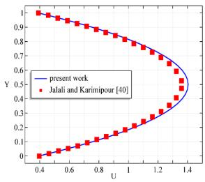
**Fig. 2** Dimensionless velocity profile at the vertical line X = 0.6L for input Reynolds number Re = 10,  $\emptyset = 0.02$ , B = 0.1, and injection Reynolds number of 1.
