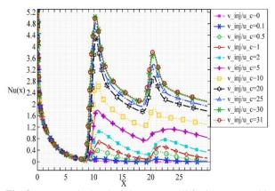
Fig. 8 Nu<sub>x</sub> calculated on the upper wall for input Reynolds number Re = 1,  $\phi = 0.02$ , B = 0.1, and different injection velocities.
