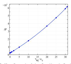
**Fig. 10** Pressure drop for input Reynolds number Re = 1,  $\phi = 0.02$ , B = 0.1, and different injection velocities.
