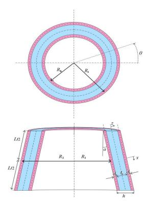
Fig. 2 Geometrical parameters of conical composite sandwich shell of fairing [33].
