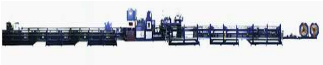
Fig. 1. Automated line for the welding of fin tubes by high-frequency welding machine.
