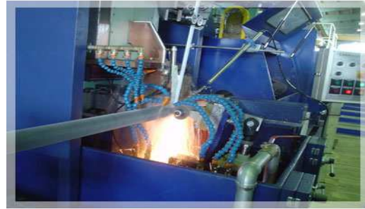
Fig. 3. The welding process currents of high frequency.
