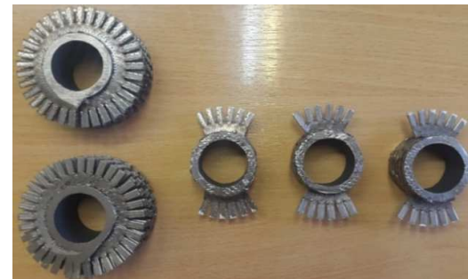
Fig. 5. Sample preparation of Finned Tubes Welding (metallography, tensile strength and hardness tests).
