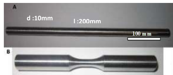
Fig. 3. a) After Machining b) Fatigue Sample.
