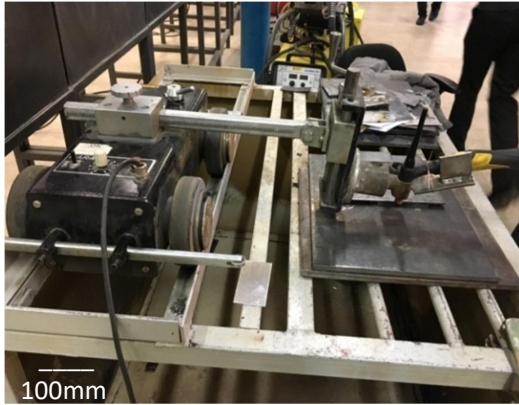
Fig. 3. PEG1 Tractor welding robot.
