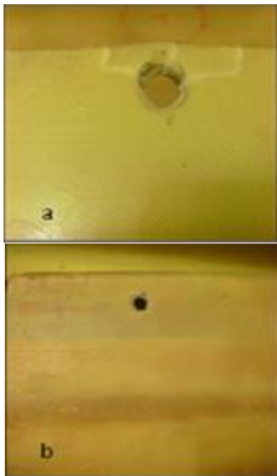
Fig. 4. Hybrid composite after loading on a.sample2 , b.sample3 without any fracture.
